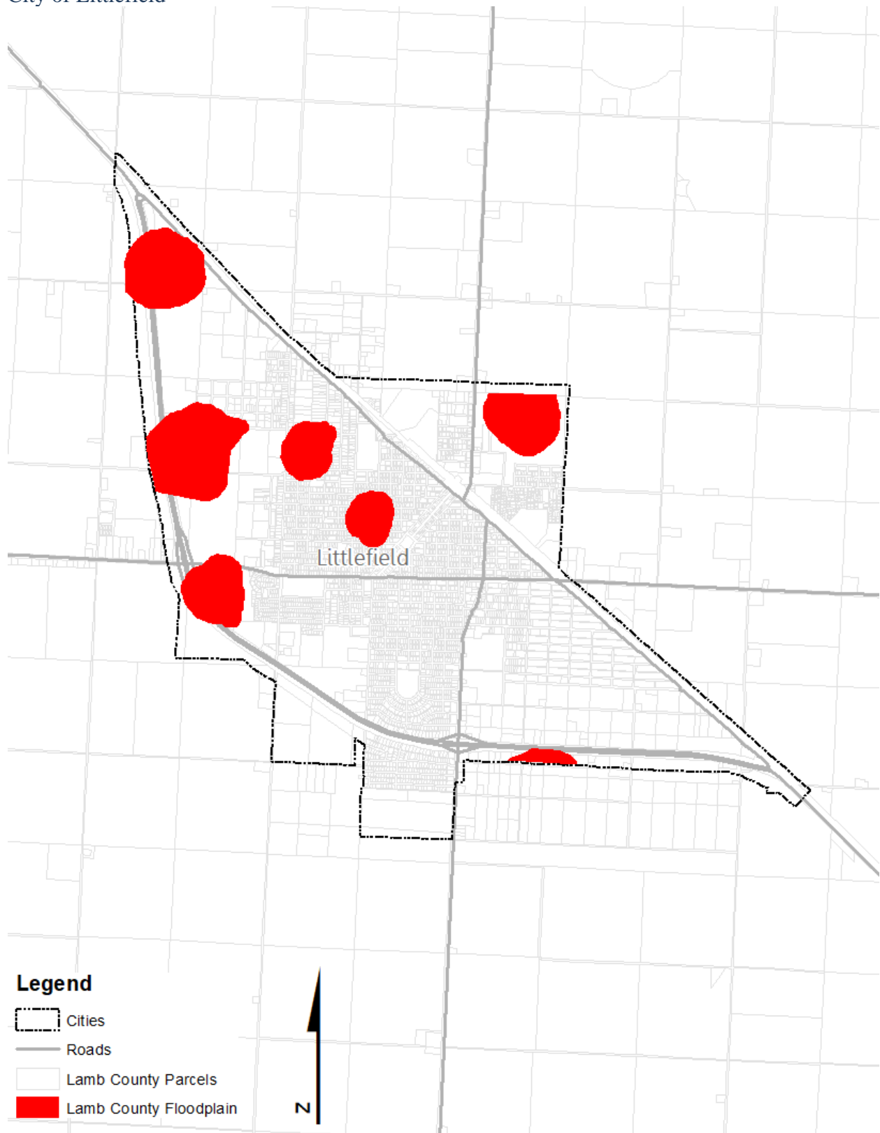
Figure 7: City of Littlefield FEMA Special Flood Hazard Areas
